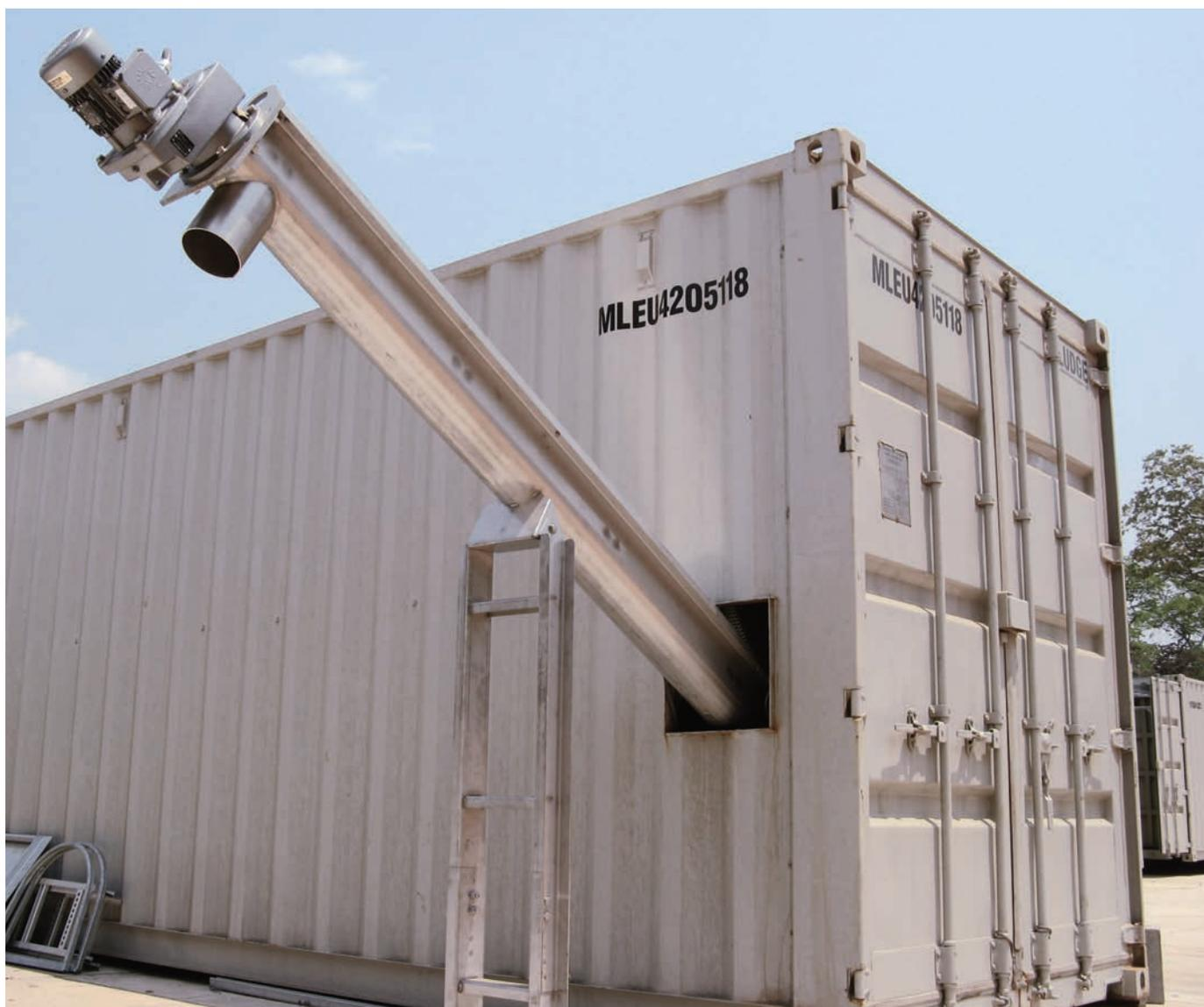
**Large Capacity System Features Integrated Sludge Thickening and Dewatering Equipment.**
